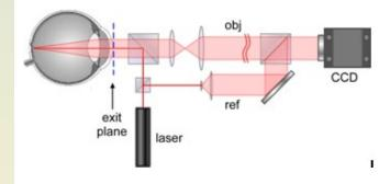
Illustration of the Ophthalmic Imaging System — Digital Holographic Adaptive Optics (DHAO)
