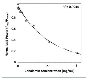
Proof of Concept that the Device Can Detect an Analyte (Cobalamin) in a Sample
