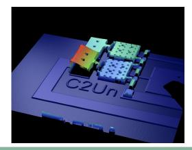
Pop-up mechanism with anchored fulcrum. The flexible hinged design reduces the pull-in voltage, while allowing spatial separation of wanted and unwanted portions of the output spectra.
