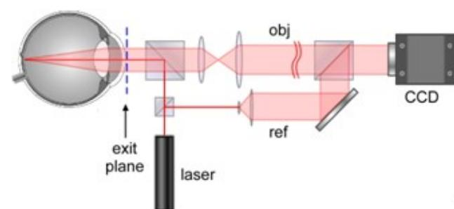
*Illustration of the Ophthalmic Imaging System — Digital Holographic Adaptive Optics (DHAO)*
