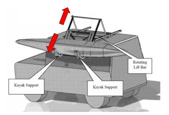
The roof rack on a vehicle while actively loading a kayak. The supports fold, storing the cargo on the roof.
